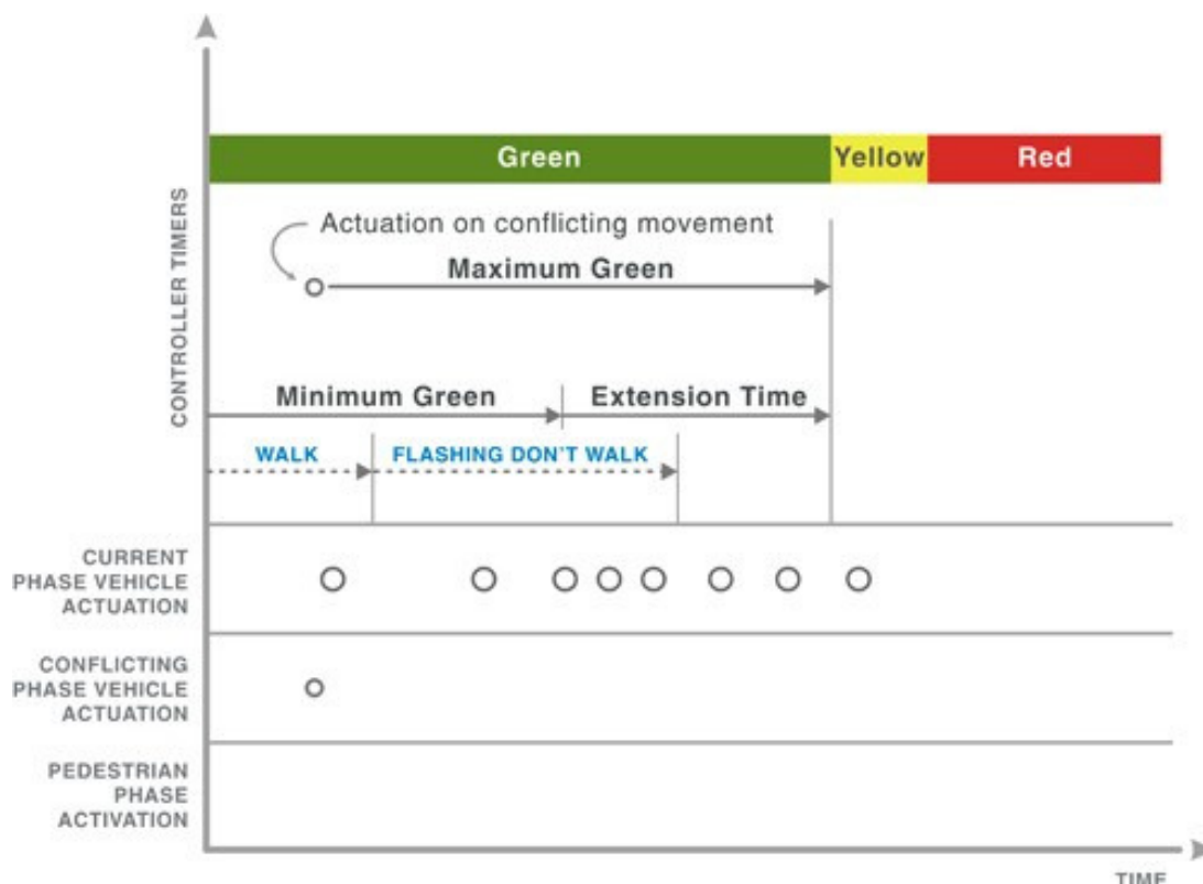
Figure 33.22-2 Settings that define the duration of a vehicle phase
